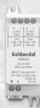
A2D0001 is a BLE-enabled 2 channel 0-10V or DALI controller. It has a universal 100-277V AC input voltage range and can control 2 separate analog channels, 1 Tunable White channel, or one Dali channel.
