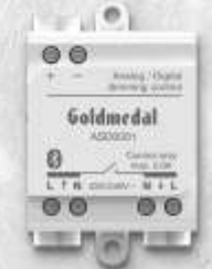
ASD0001 is a BLE-control unit for LED drivers with 0-10V, 1-10V, or DALI dimming interface. The control output can be configured either as analogue 0-10V (and 1-10V) or as a digital standalone DALI control interface.
