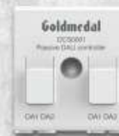
DCS0001 is a BLE-enabled DALI controller. It does not have its own power supply. Instead, it is powered directly from a DALI bus. DCS0001 can be used with a DALI sensor for presence detection or daylight harvesting or it can be used for controlling Human Centric Lighting (HCL).
