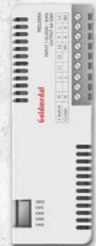
REL0004 is a BLE enabled 4 channel relay with 4 separate inputs to control BLE device on the network. The 4 inputs can be freely programmed to do operations like Dimming, curtains, master functions etc. The device can be used for curtain control also.
